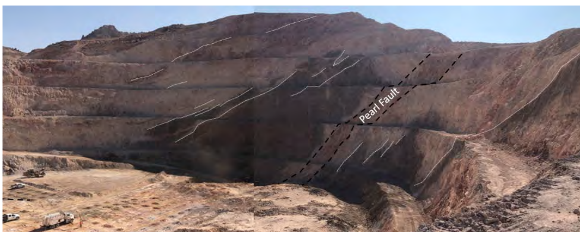
Figure 13-2 View looking South in the Pearl Pit showing continuous, moderately to shallowly-dipping shears of the Pearl Fault
